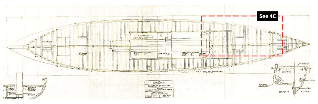
NOTE: December 1992 Hull Framing Plan from *Minnehaha* Restoration (1990-1996). Construction of the hull's framing has not changed since restoration.
