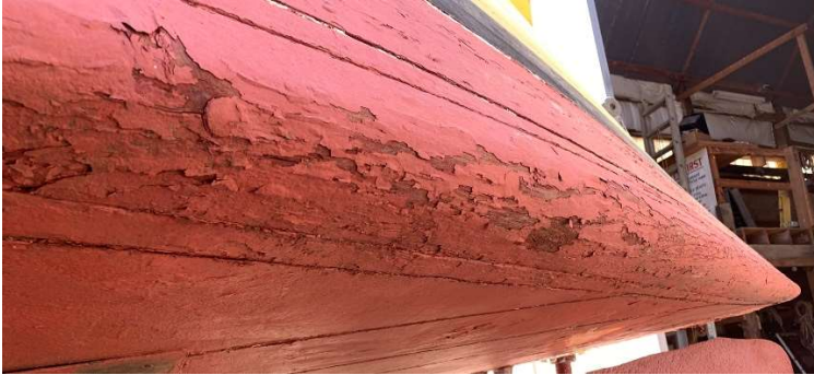
Current state of the old bottom paint tht needs to be removed
